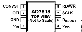
Figure 5. AD7818 Pin Configuration
